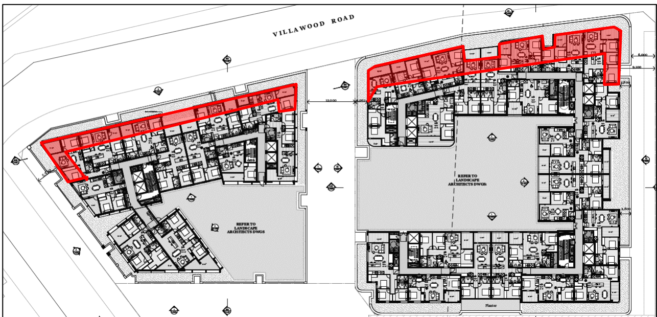
Figure 5-2 Traffic Intrusion Requirements for Glazing (Level 3,4&5) – Zone A in Red
