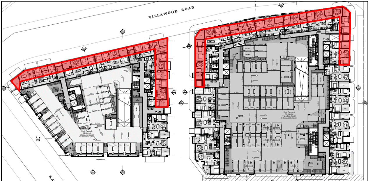
Figure 5-2 Traffic Intrusion Requirements for Glazing (Level 3,4&5) – Zone A in Red
